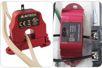
5. Lock the Current Loop closed by pressing the cover down firmly and listening for the click.
